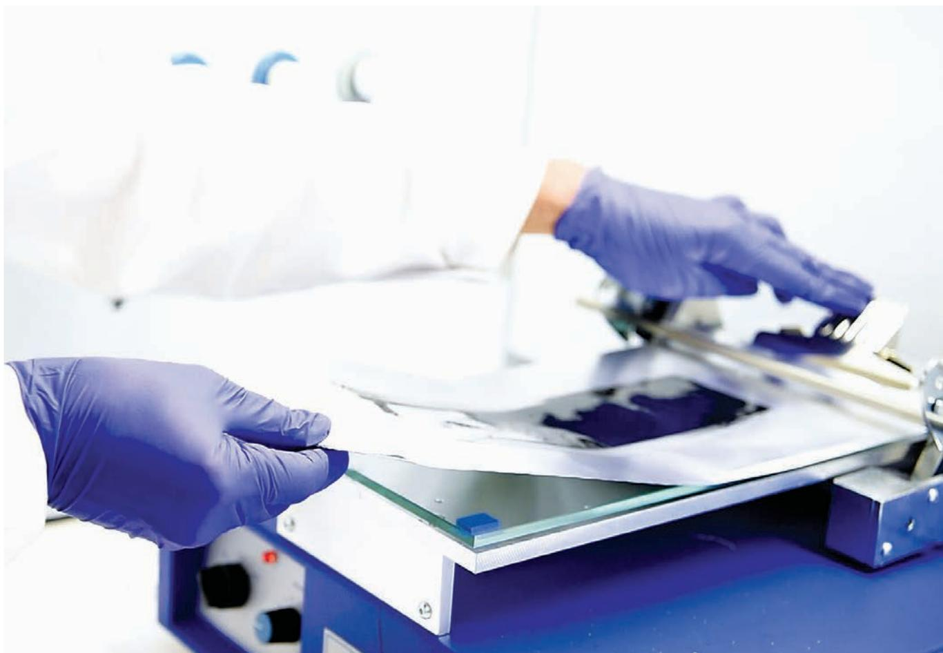
A researcher uses a manual draw-down coating process to prepare small-scale electrode foils at BatTRI-Hub.
