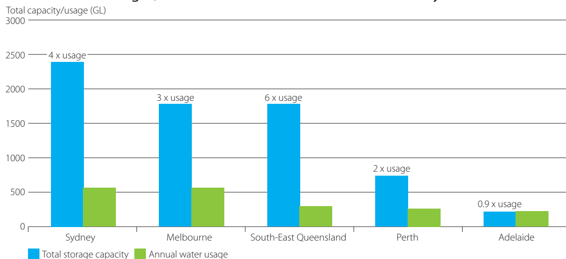
Figure 5.6 Total storage capacity and annual usage for mainland State capitals. Sydney's reservoirs, once full, can supply up to for years' consumption. Adelaide has much smaller storages, as it can draw water from the River Murray.
