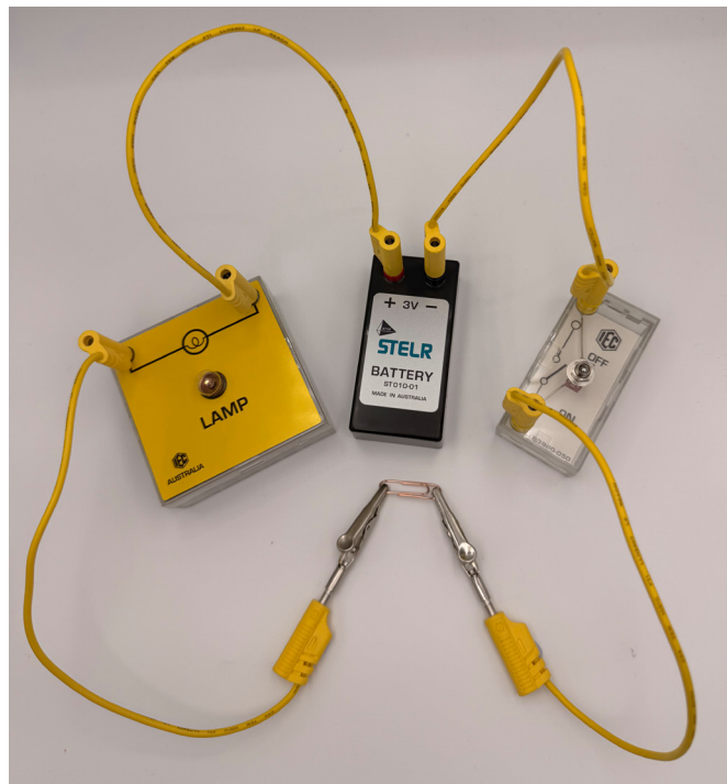
Above: Example setup of a circuit for testing materials
