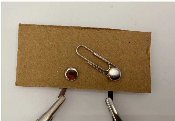
Above: The switch is open
