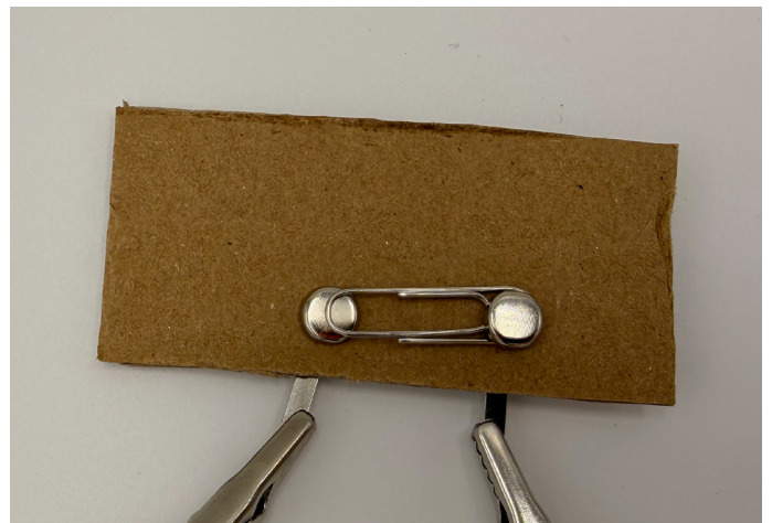
Above: The switch is closed
