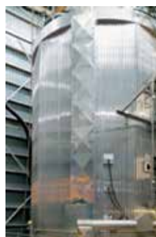
Figure 9 Vertical drier reactor for the Barwon Water Bioprill® plant.
